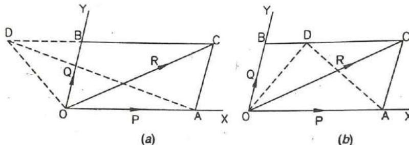
Let P and Q be any two forces acting at a point O along lines OX and OY respectively and let D be any point in their plane as shown in Fig 1.44.
