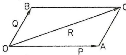
**DETERMINATION OF THE RESULTANT OF TWO CONCURRENT FORCES WITH THE HELP OF LAW OF PARALLELOGRAM OF FORCES**
