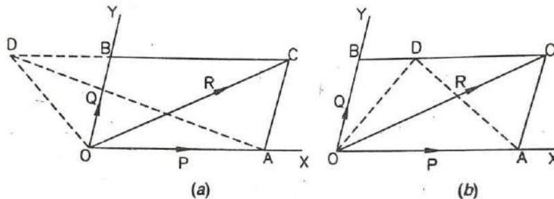
Let P and Q be any two forces acting at a point O along lines OX and OY respectively and let D be any point in their plane as shown in Fig 1.44.
